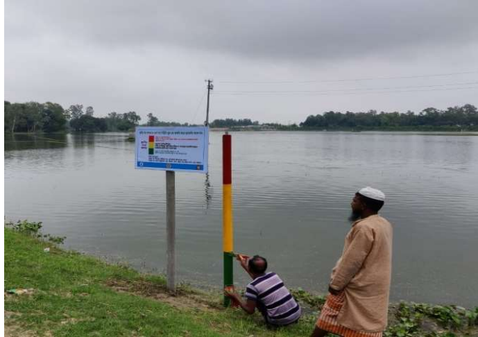
Flood markers were installed at Tekani Union of Kazipur Upazila.
